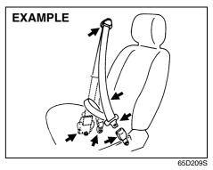
Adjust the shoulder anchor height so that the shoulder belt rides on the center of the outside shoulder. To upward, slide the anchor up. To downward, slide the anchor down while down the lock lever. After adjustment, make sure that the anchor is securely locked.
